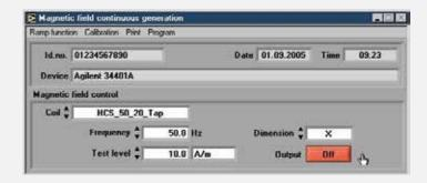
Open the continuous generation window for long term magnetic field test.
