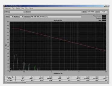
Open the Magnetic field measurement window for spectrum analyzer measurements. Perform a single or continuous measurement. Perform test according to predefined standards.
