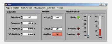
The software starts with the generator/amplifier control panel. This window allows basic settings of generator and amplifier.
